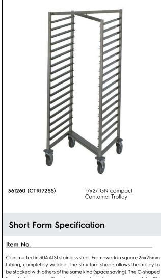
"non-tip" runners, with upturn at each end, can accommodate GN containers 2/1, 1/1, 1/2 and 1/3. N. 4 swivelling castors, two with brakes, mm125 in diameter, fitted with plastic bumpers.
